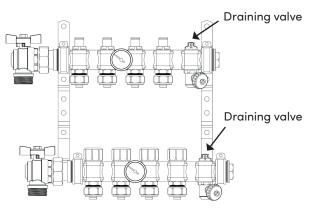
tem, there is poor, or no, circulation of the water, which for the underfloor heating system in particular results in heat only being available up to the flow loop of the manifold, while the return loop is cold, or maintains the current room temperature.
