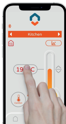
The temperature is easily adjusted by sliding the temperature indication up or down.
