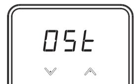
3- The display indicates to you the measured temperature correction value (which is 0 by default).
