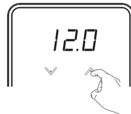
3- The setting is active after a few seconds and the thermostat will return to the main screen.
